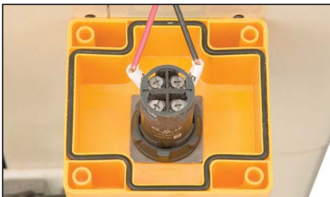
Figure 89. Rear emergency stop button wiring.
